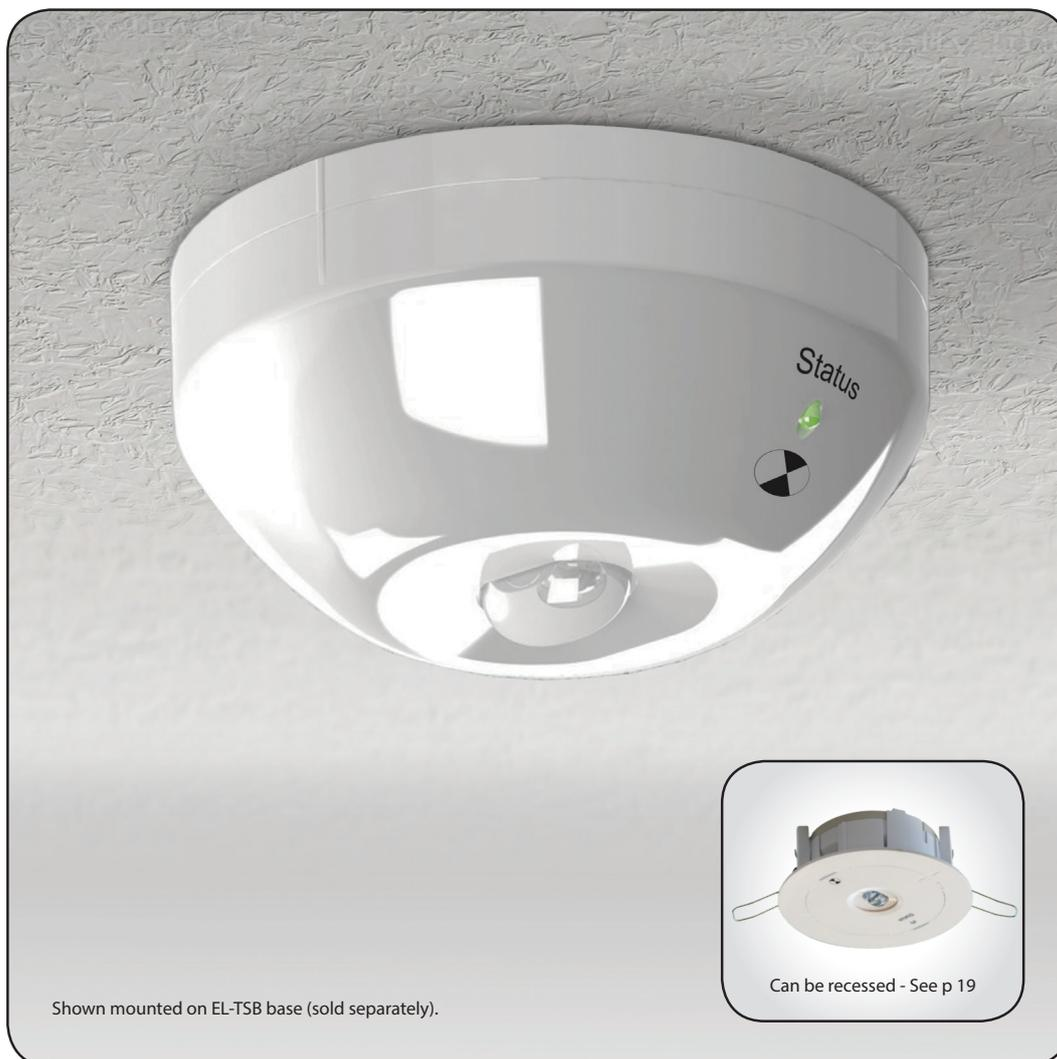
EL-DL2-AS is an LED-based, addressable corridor down light featuring one high-powered LED with a specially engineered dual surface free-form optic. The unit's body contains the electronics and the stand-by battery and features a bicoloured status LED indicating charge/fault status (green for charging, red for fault).
